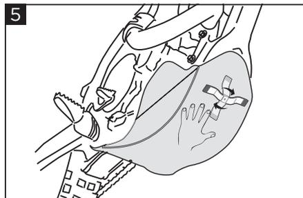
**5 Push the skid plate and screw 90° the bracket (B).**
