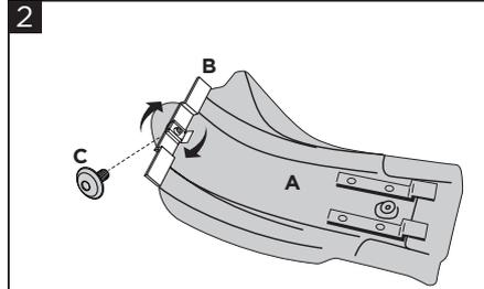
**2 Screw two turns the screw (C) on the bracket (B).**
