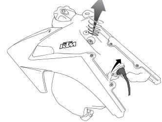
**Unscrew the seat screw. Disconnect the fuel pump power cable.**
