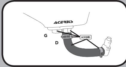
**3. Install the Acerbis pump line and use the acerbis retaining clips.**
